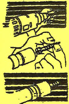
**Instructions for use:** Using a 3/16" drill bit, drill a hole a minimum of 1/4" deeper than the maximum embedment depth of the anchor (minimum anchor embedment should be 1"). Place the anchor through tread into the pilot hole and drive in with Phillips bit.
